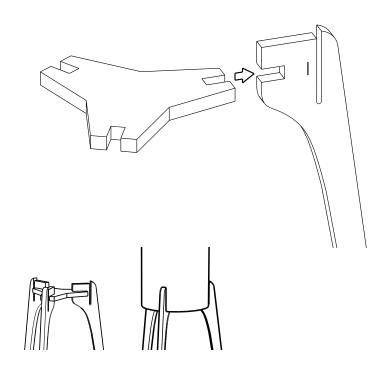
Push the connector plate onto the leg until it reaches the vertical line stop mark adjacent to the slot.
