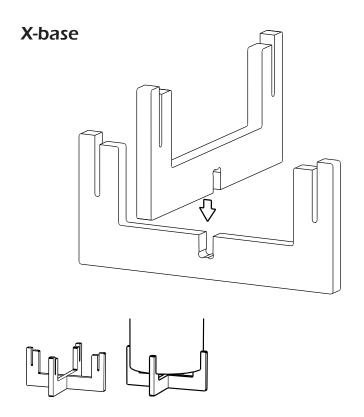
Push the two base pieces together until the bottom faces align.
